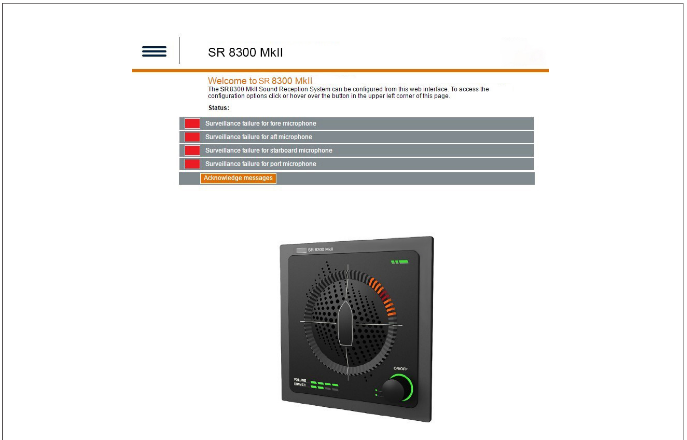
Figure 30: Home screen, status Failed - Acknowledge messages
