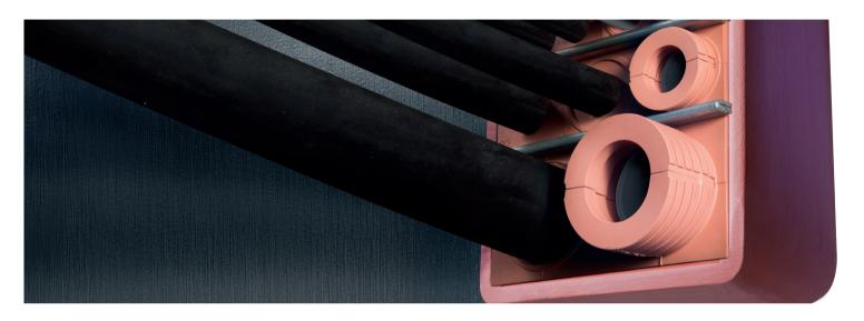
By installing a HandiPlug in the HandiBlock, you can quickly and easily create a spare block. This is a fully certified way to prepare for future cabeling/piping. HandiPlug's low weight and smart design, together with HandiBlock, create a secure pressure-tight unit. The plug's unique design also acts as a circular former for the sealing insert. Rather than being compressed and deformed into an oval shape, the plug enables the InsertStrip to retain its roundness even
