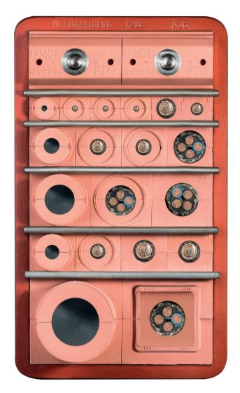
The HandiBlock is a new safe, flexible and easy-to-install insert block. The sealing range is now fully adaptable to the cable/pipe diameter, within the module size. If a cable/pipe is scheduled or installed after the initial installation, safe installation can be achieved by using a reusable block. In this case, a main block, InsertStrip and HandiPlug can be assem-
