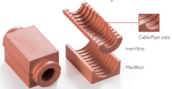
The HandiBlock is available in four sizes to fit cables and pipes or tubing from 4 to 54 mm. A HandiBlock consists of two compact half MainBlocks and two InsertStrips. Every compression ring on the InsertStrip has clear markings to indicate different cable/pipe diameters. This helps the installation technician to quickly and safely identify the correct size of the MainBlock, InsertStrip and compression ring.
