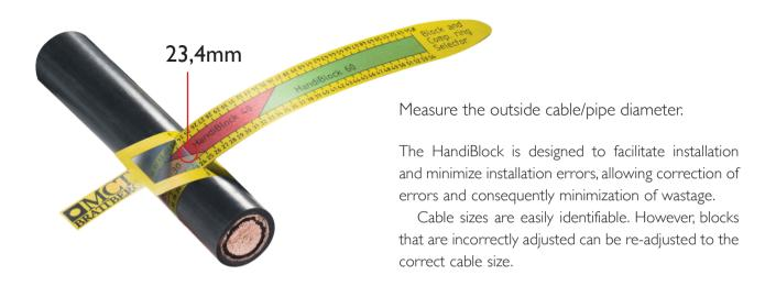
To choose the size of the compression rings from the InsertStrips, use the rings closest in size, over and under, so that the measured cable size is **in between**. For cable size 23,4 mm, the rings will be 23 mm and 24 mm.
