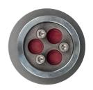
The MSR cable gland consists of a steel housing with screw thread, a gasket, a sealing nut and a filling element. The filling element is made of silicone rubber and finished with steel mounting parts. The rubber of the MSR cable gland consists of a core, or a few cores, and 1 or more round rings, which can be removed in order to be able to properly seal the cable (s). If the core is not removed, the MSR cable gland can also be used, partially or completely, as a blind lead-through.
